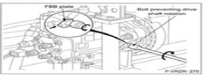
(16) Loosen the bolt preventing drive shaft rotation, install the FBB plate and fix the FBB plate by tightening the bolt preventing drive shaft rotation.
