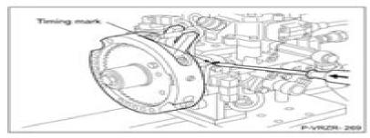
(15) Mark the timing mark on the injection pump and the bracket.
