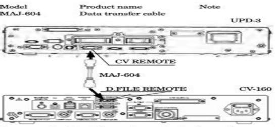
For connecting the video system center to the endoscope position detecting unit, use the
