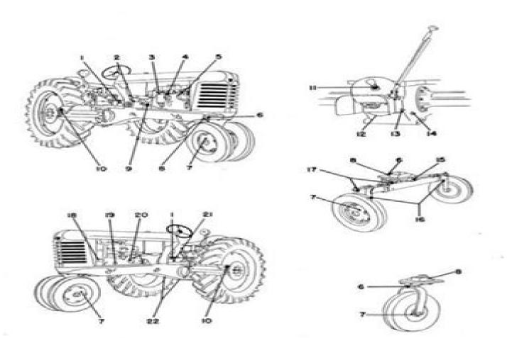
Figure 1-1 Now Crop Lubrication Diagram
