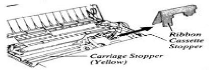
When you transport or ship the typewriter, be sure to position the carriage at the far right of the unit, and insert the Carriage Stopper and the Ribbon Cassette Stopper.
