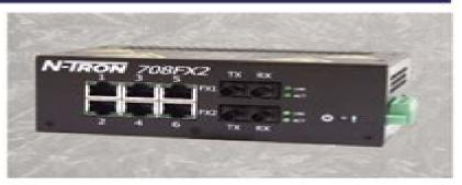
Rapid Spanning Tree - This function allows the switch to be configured in a Ring or Mesh topology, and provides support for redundant path communications with high speed (rapid) healing.
