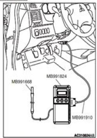
To prevent damage to special tool V.C.I. (MB991824), always turn the ignition switch to the "LOCK" (OFF) position before connecting or disconnecting special tool V.C.I. (MB991824).
