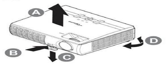
To raise the level of the projector, lift the projector [A] and press the height-adjuster button [B].
