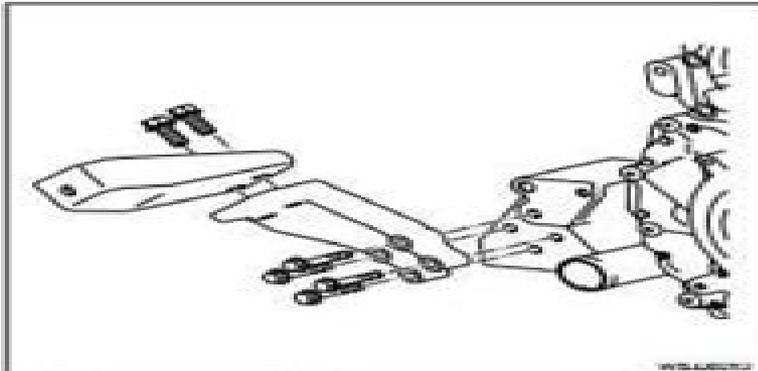
5. Remove the bolt with arrow mark which holds the water intake pipe to the engine foot RH.
