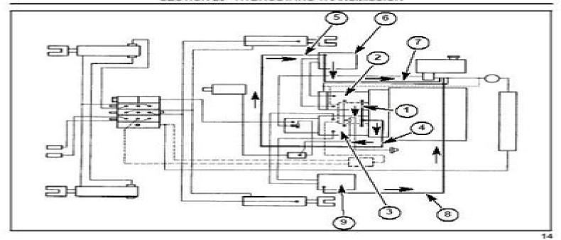
Hydrostatic Pump and Motor Case Drain Flow (LS180 and LS190 Two-Speed Shown)
