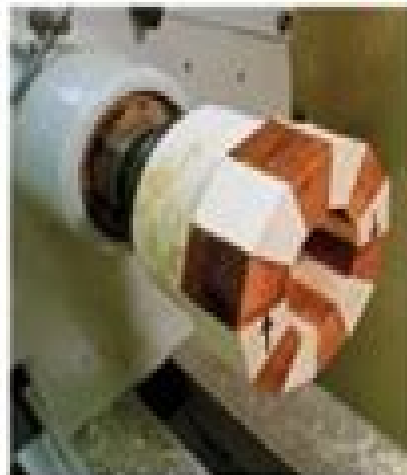
Figure 3-18: Ring mounted on the lathe with two hands off and smooth ends
