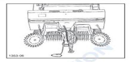
A GREEN-FEED KIT is available for all three models. It consists of extra tines for the windguard that keep greener or unconditioned crops from spearing up into the rolls.
