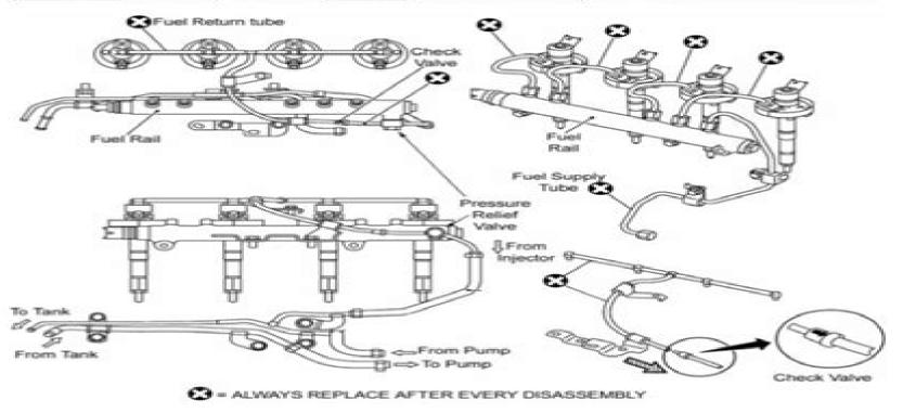
NEVER "CRACK OPEN" AN INJECTOR LINE WITH THE ENGINE RUNNING OR CRANKING.
