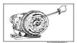
TIGHTEN THE TORQUE CONVERTER AND THE ADAPTER. Tightlening Torque: 33.5-38.5 N m (343-392 kgf cm, 25-28 lbf ft)
