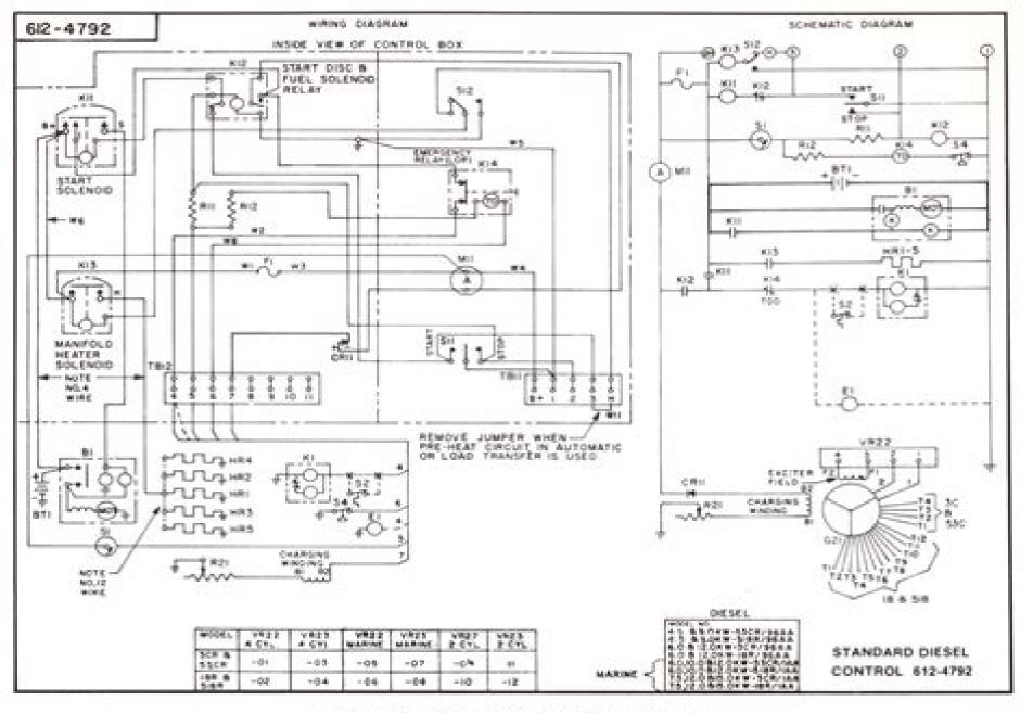
FIGURE 5-16. DIESEL GENERATING SET CONTROL
