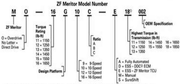
Progressive torque is an engine feature that requires a Torq-2 transmission. In models not featuring progressive torque, this number will be the same as the torque rating.
