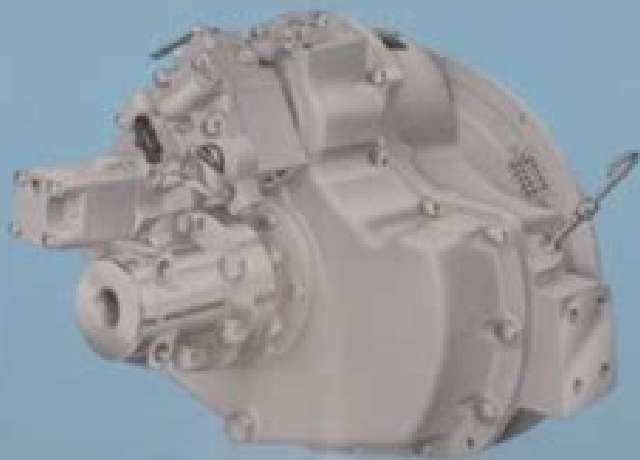
MG-507-1 with Optional Trolling Valve and Companion Flange
