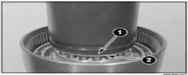
Install the CNH 299026 Bearing Puller Tube over the shaft, turn the screw counterclockwise until the open end of the tube (1) contacts the clutch spring retainer (2).
