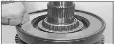
Remove the pressure plate retaining ring.
