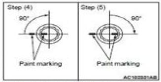
(4) Apply a paint mark to the heads of the cylinder
