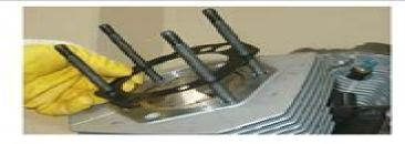
Slide off the cylinder from the stud bolts, paying attention not to damage the piston.
