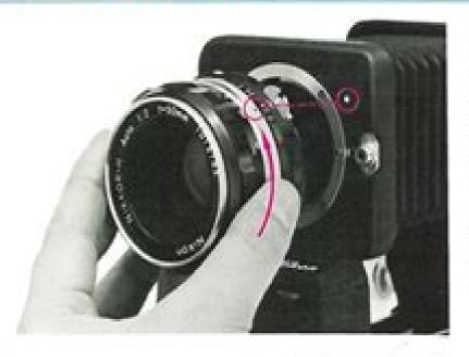
Position the lens in the bayonet mount on the lens panel, lining up the black dot on the lens with the white dot on the lens panel. Then twist the lens counterclockwise until it clicks into place.
