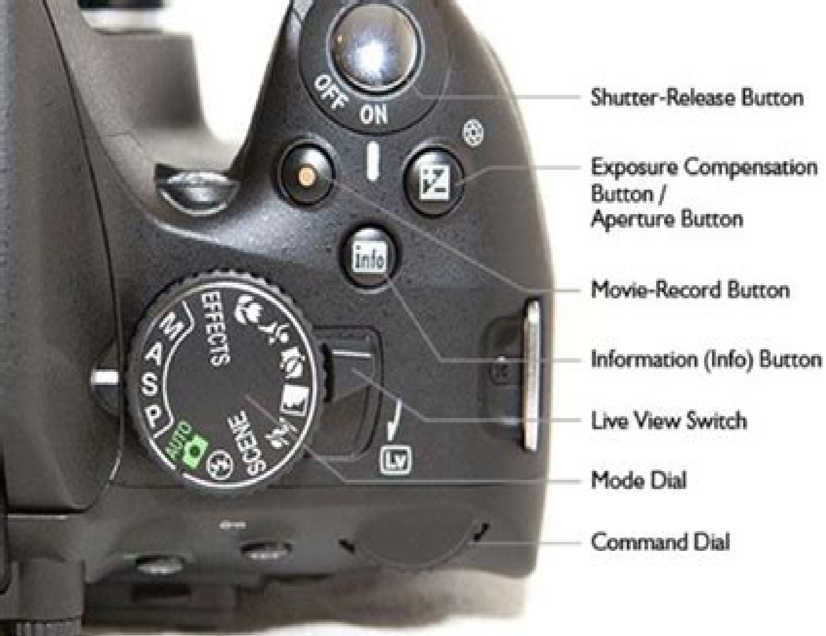
Figure 2 - Controls on the top of the D5100
