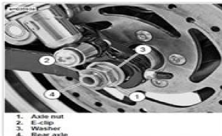
Figure 2-11. Rear Wheel Mounting
