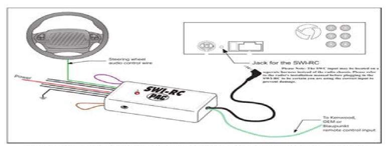
For Alpine, Clarion, JVC, Pioneer, Sony or Valor radios, connect the SWI-RC 1/8" plug into the radio's Steering. Wheel input jack on back of radio or wire harness. For Kenwood or OEM radios, connect the blue/yel wire to the remote Input wire (blue/yel or yel/blu for Kenwood, gray for OEM) of radio.
