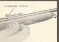
The all-purpose stock on your Remington rifle is designed for use with telescope or receiver sights as well as factory open sights. Location of rear sight holes is standard for most target telescope mounts. If rear sight is removed for receiver sighting clearance, receiver plug screws, in top panel of receiver, may be used to fill rear sight barrel screw holes.
