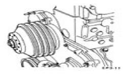
Remove the fan bracket assembly (except crane).
