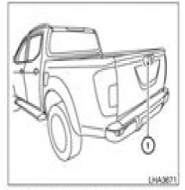
To display the rear view, the RearView Monitor system uses a camera located next to the tailgate handle (1).
