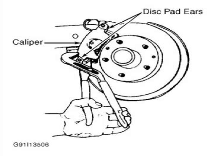
Fig. 2: Bending Outer Pad Ears Toward Caliper Courtesy of GENERAL MOTORS CORP.
