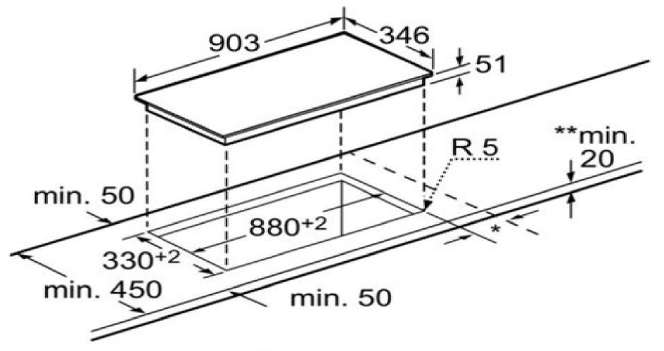
\* The minimum distance from the hob cut-out to the wall is 40mm
