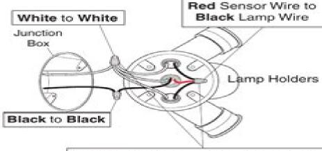
Optional: Connect additional load across the white and red wires. Total lighting load including lampheads on fixture must not exceed 500W (4.2A).
