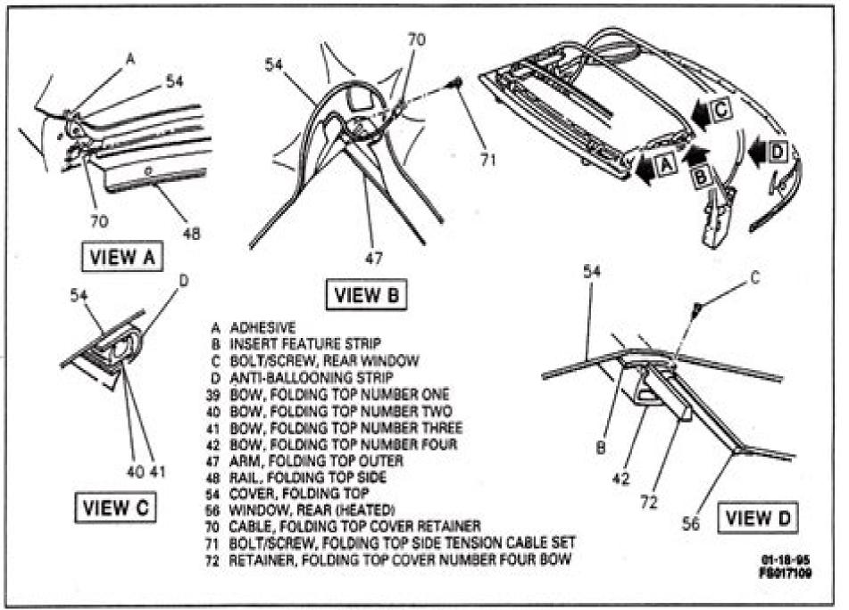
Figure 17 - Top Cover Fastening Details
