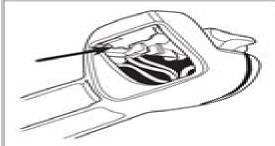
The stop switch can be easily detached with a screwdriver.
