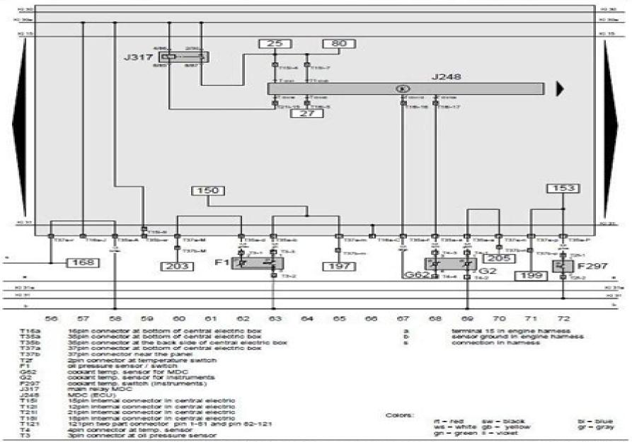
Central electric, oil pressure sensor, coolant temp.-sensor
