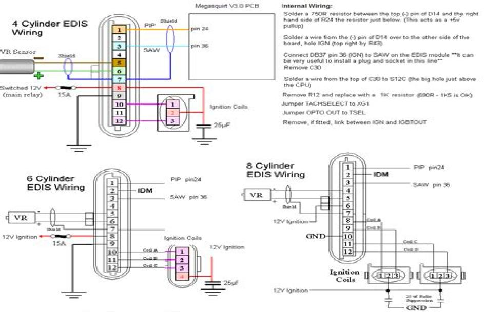
Note: The EDIS4 and EDIS8 plugs are not interchangeable - note the different guide key details.
