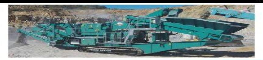
The high performance Powerscreen® Pegson 1000 Mastrak is a small to medium sized cone crusher. which has been designed for direct feed applications without pre-screening on dean rook. At its heart is: the Automax<sup>a</sup> cone crusher which provides excellent reduction and product outlicity for the production. of high quality appreciate and auto-base material. Hydraulic release capabilities are designed so that any uncrushable material entering the chamber is safety discharged.
