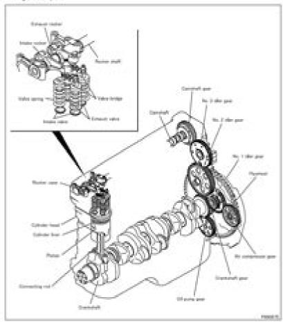
The BRSGTs engine employs an overhead samuhal (CHC) system, with the valve mechanism and the timing great emerged as shown above.
