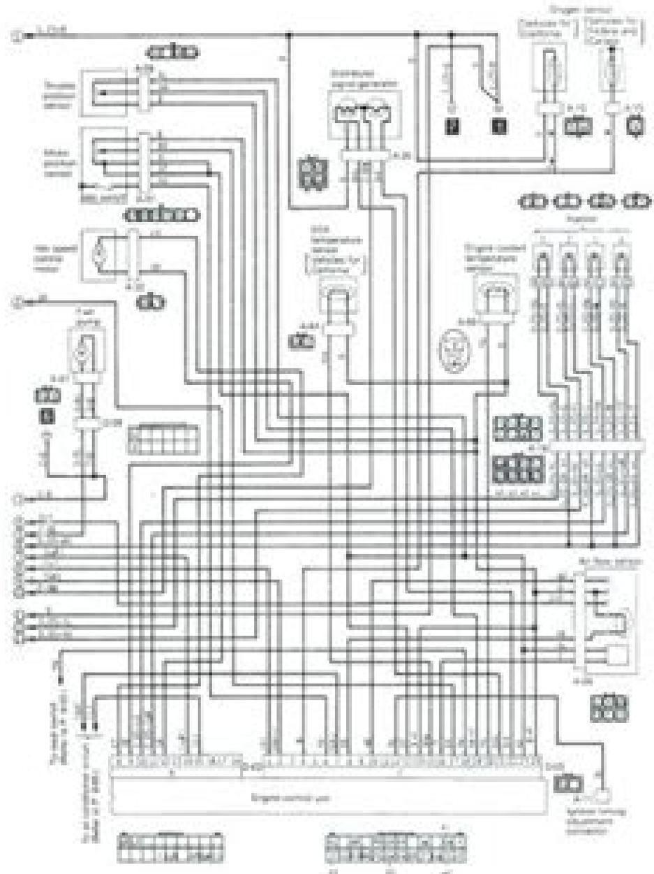
20.11b Fuel injection circuit (2.4L engine - 2 of 2)
