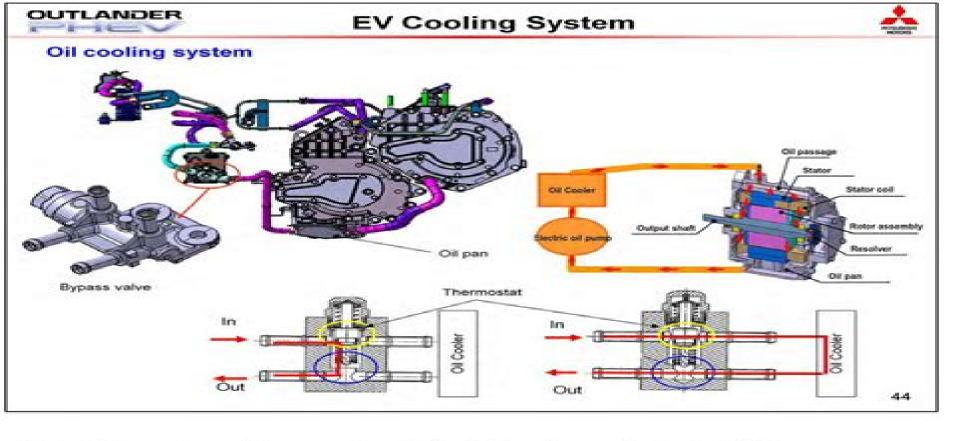
Motor / Generator coil temperature's limitation: Approximately 120°C
