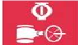
Automatic Sprinkler Control Valve
