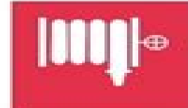
Fire-Fighting Hose or Standpipe Outlet
