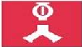
Fire Department Automatic Sprinkler Connection — Siamese
