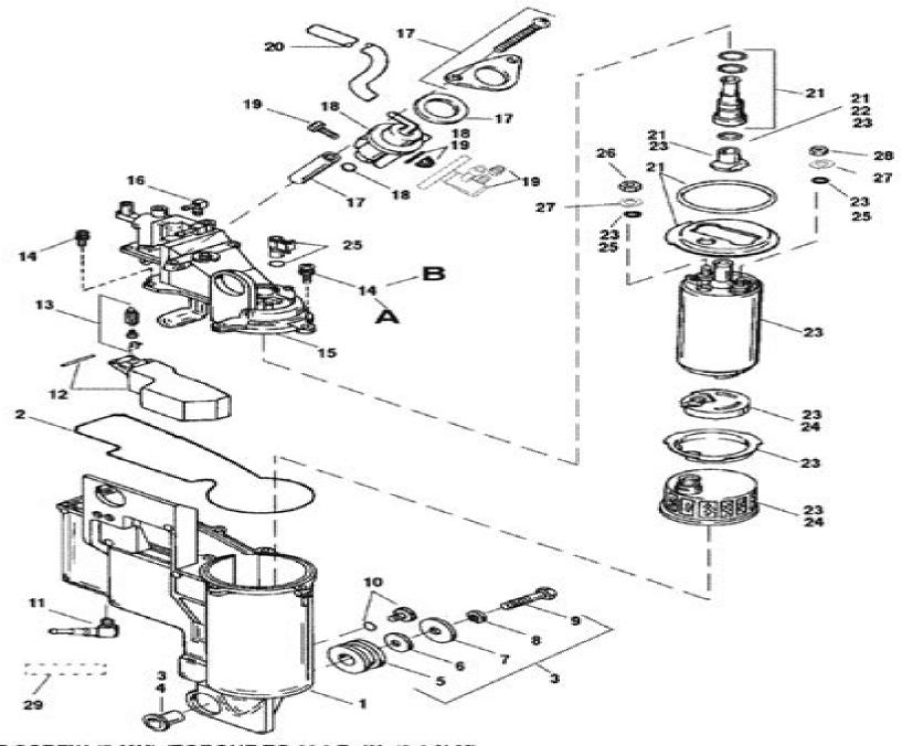
A = LARGE SCREW (5 MM) (TORGUE TO 30 LB. IN. (3.4 N.M) B = SMALL SCREW (4MM)(TORQUE TO 20 LB. IN. (2.3 N.M)
