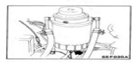
3. When fuel overflows, retighten and connect fuel filter sensor.
