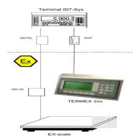
Operation and Display of Weightvalues and Scale-Functionsfor the EX-Zone 1.
