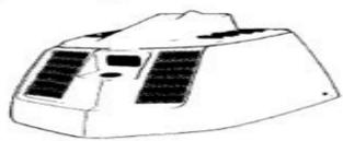
When operating the vehicle in powder snow it is advisable to block the front hood louvers as per illustration using snow deflectors supplied with vehicle. Unblock the louvers as soon as snow condition becomes firmer or as soon as engine becomes too hot.
