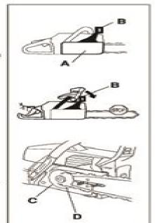
2 The front hand guard is not designed solely to activate the chain brake. Another important safety feature is that it prevents the chain from hitting your left hand if you lose your grip on the front handle.
