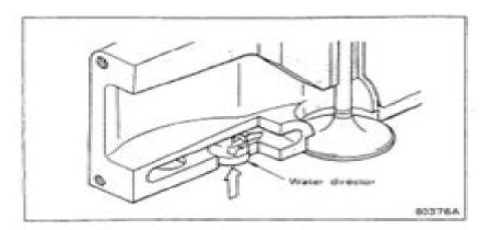
For more effective cooling of the combustion chamber, water directors which direct coolant flow are pressed into the bottom of the cylinder head.
