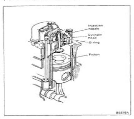
The combustion chamber is made up of the cylinder head and piston top. The injection nozzle as well as the nozzle tube is mounted to the cylinder head. The nozzle tube holds the nozzle in position and protects the nozzle sheathed by it from coolant. Since the outside of the nozzle tube is exposed to the water jacket, the top end of the tube is sealed off with an O-ring and the bottom end staked to prevent entrance of water.
