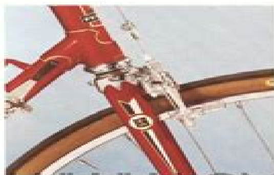
Mounting of the Mafac Racer front brake in the UO 8.
