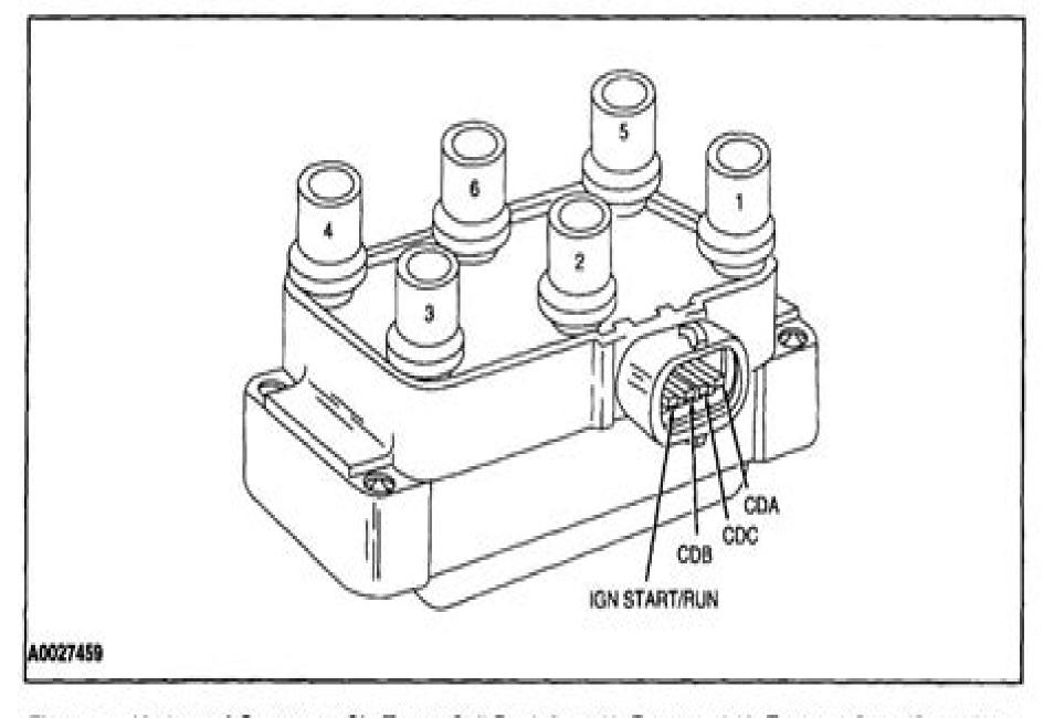
Figure 59: Horizontal Connector Six Tower Coil Pack for 4.0L Ranger, 4.0L Explorer Sport/Sport Trac and 4.0L Explorer/Mountaineer
