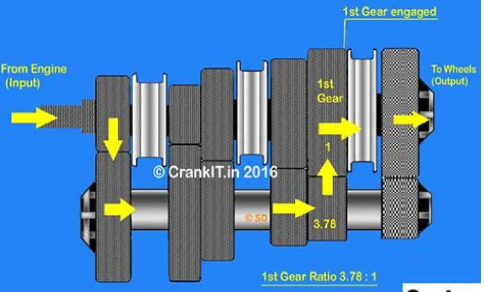
3.78 rotations of input shaft = 1 rotation of output shaft
