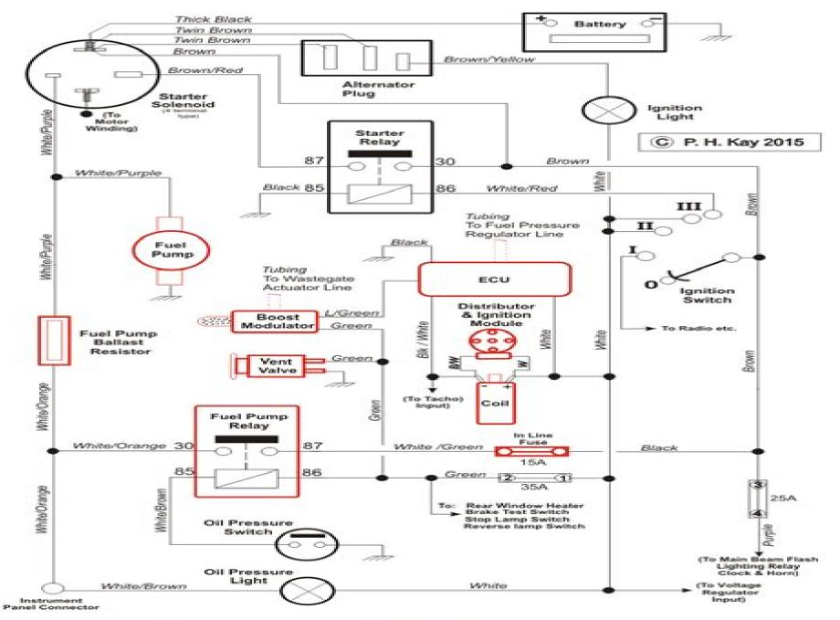
Wiring Diagram of ERA Mini Turbo Installation
