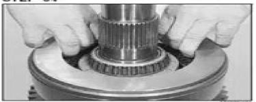
Remove the pressure plate and the eleven clutch plates.
