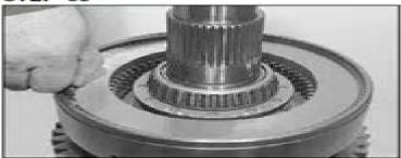
Remove the pressure plate retaining ring.
