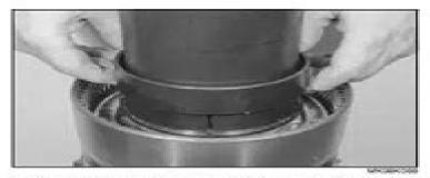
NOTE: The CNH 299026 Bearing Puller has two sets of split collars for two different size spring retainers. The correct size for each spring retainer will fit as shown.
