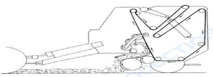
The PICKUP feeds material back to the floor roll. The WINDGUARD holds material for positive feeding. The FLOOR ROLL feeds material to the BELTS, which move material to the core-forming area. The FORMING ROLLS assist in curling the material and starting the core. When the bale reaches a predetermined size, the wrapper engages automatically.
